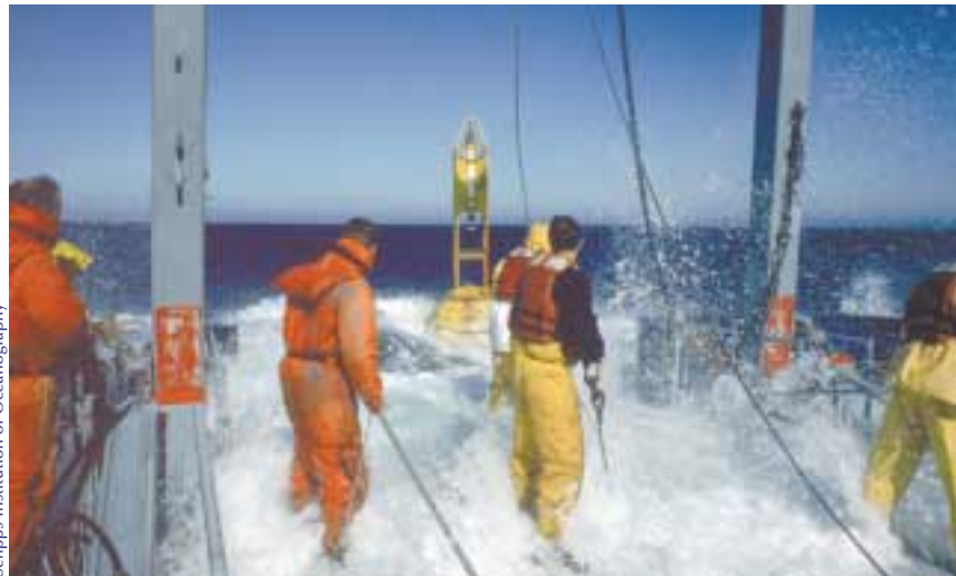
High seas wash onto the deck of Scripps Institution of Oceanography's research vessel New Horizon as scientists work to retrieve a large buoy. The 1,800-pound buoy is anchored to the seafloor by a cable that has instruments to measure underwater currents and temperature at various depths.
